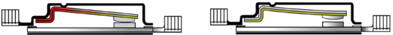
The more sensitive the bimetal, the more quickly the circuit will be opened
